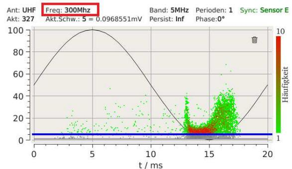
Figure 2 PRPDP at 300MHz centre frequency
