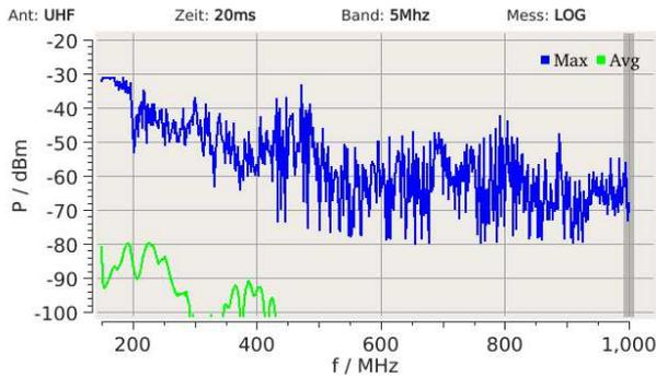
Figure 3 Spectrum of surface discharge
