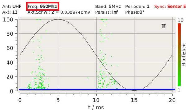
Figure 4 PRPDP at 950MHz centre frequency
