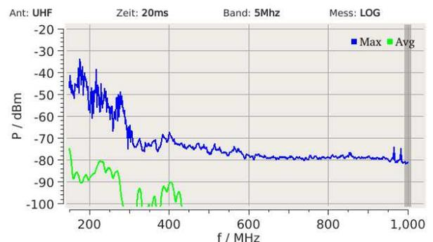
Figure 7 Spectrum discharge in large void
