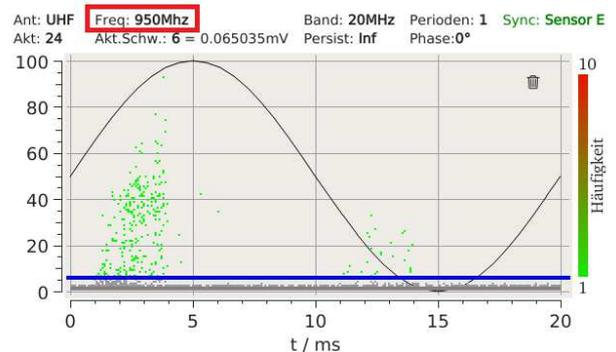
Figure 6 PRPDP at 950MHz center frequency
